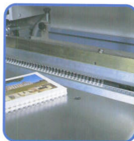
The wire in the tool ready for binding.
