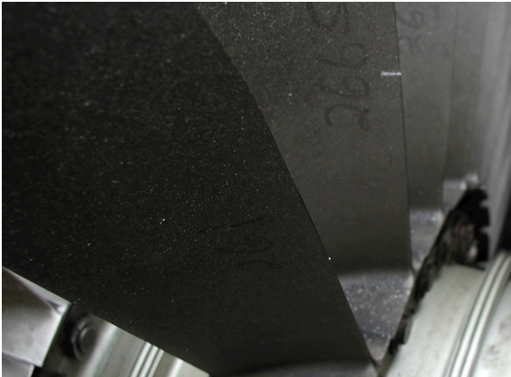
Figure 7: Damaged blade (Number 2) fitted to engine
