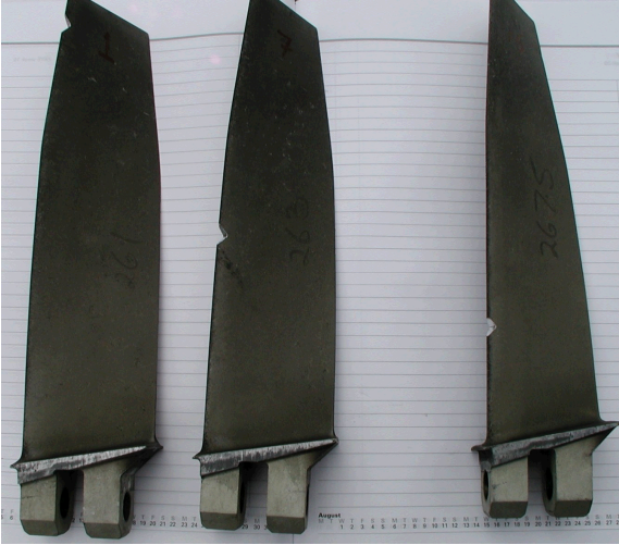
Figure 6: Damaged blades (Numbers 1, 7, 15) fitted to engine
