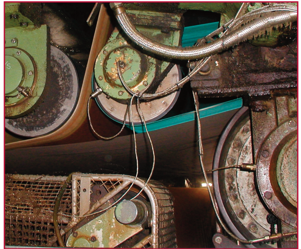
TWO STUD MOUNTED ACCELEROMETERS ATTACHED TO ONE OF THE MACHINES AT ST REGIS' KEMSLEY MILL.
