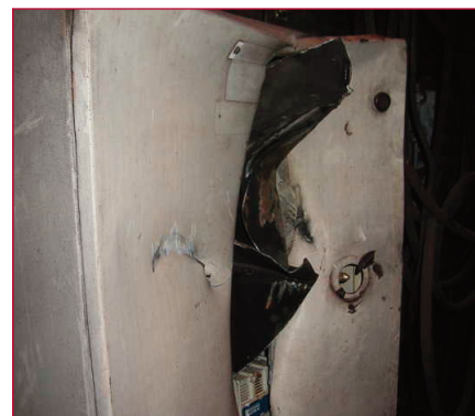
An impellor blade thrown from a fan ended up embedded in a control panel, but with a predictive maintenance strategy in place, occurrences such as this are rare.
